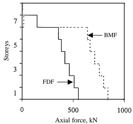
Figure 9: Envelope of column axial force
