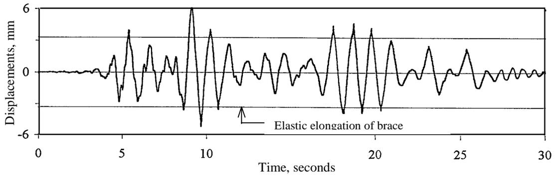
Figure 7: Time-histories of slippage in friction-damper
