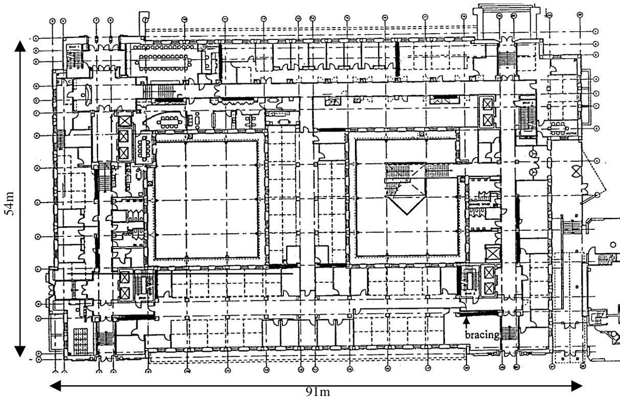
Figure 2: Typical floor plan showing location of bracing with Pall Friction-Dampers
