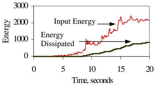
Figure 7. Energy input and energy dissipated by friction-dampers
