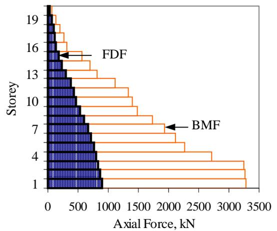
Figure 10. Envelope of column axial force
