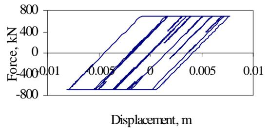
Figure 8. Hysteretic loop of friction-damper and brace
