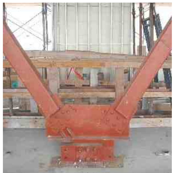
Friction damper in chevron bracing (inverted)
