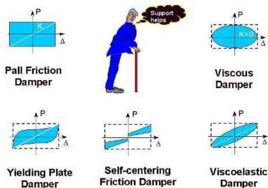
Figure 3. Comparison of Hysteresis Loops of Different Dampers
