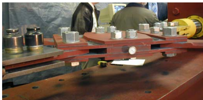
Figure -6. Friction Damper Under Testing
