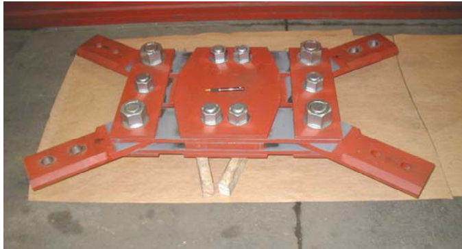
Figure-5. Friction Damper In the Lab
